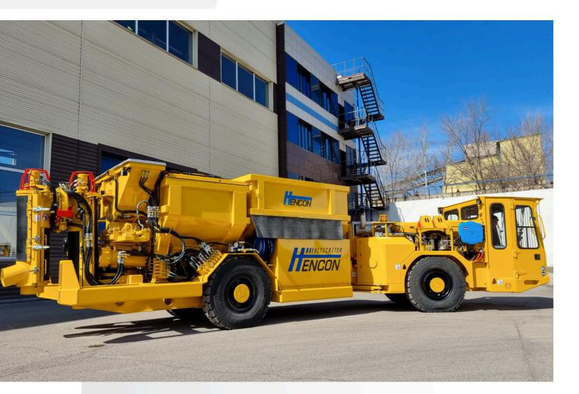
The Hencon TransVers High Profile Batch Mixer has been designed for the preparation of concrete mixtures that are used in Hencon Shotcreter machines.
